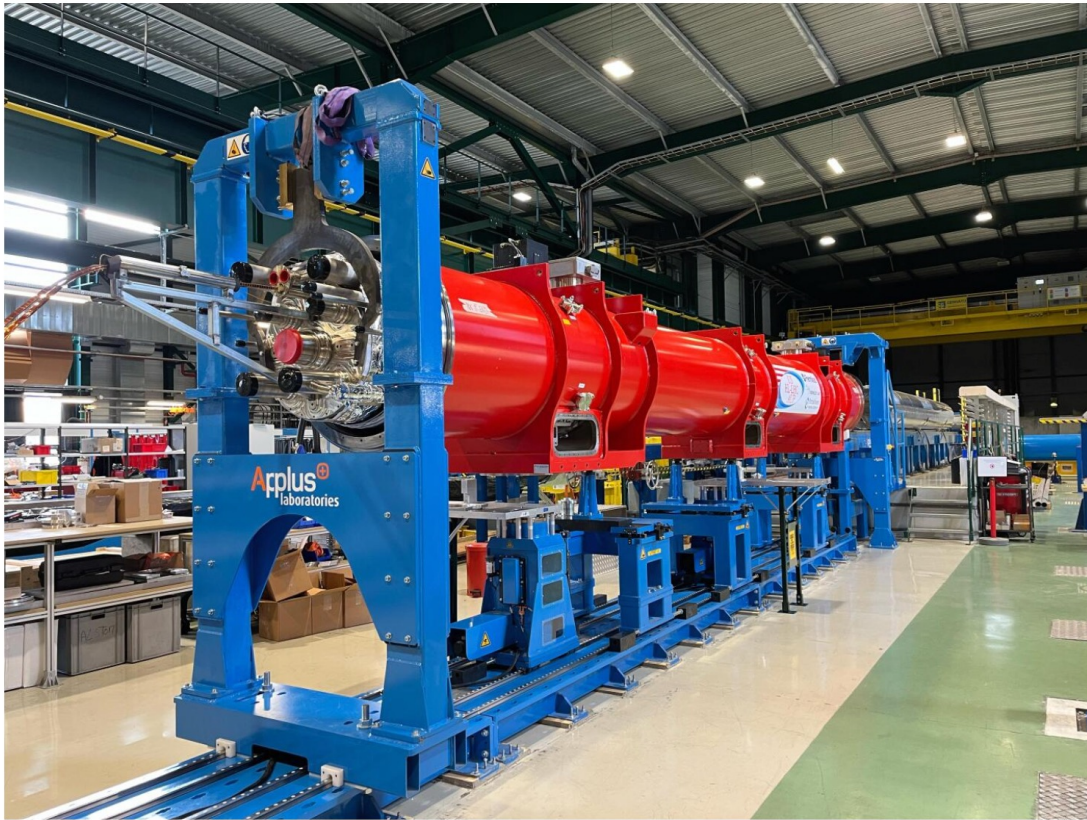
The cryo-assembly containing two MQXFA magnets was delivered to CERN in early December. (Image: CERN)
