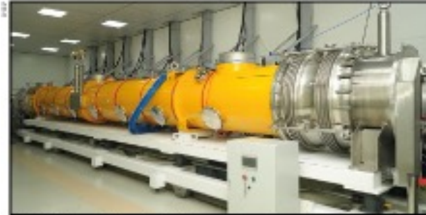
CEPC technologies A 1.3 GHz 8 \times 9 -cell cavity cryomodule (left) and a 650 MHz 800 kW continuous-wavelength, high-efficiency klystron (right) developed and tested at IHEP in Beijing.
