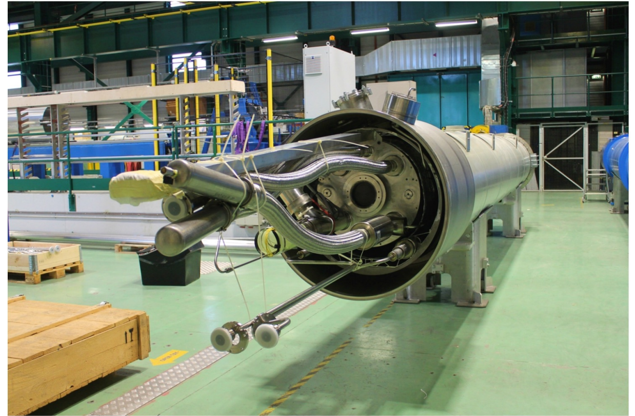
The magnet, named MQXFB03, is 7.2 metres in length. It is the first of ten that will be needed for the HL-LHC. (Image: CERN)
